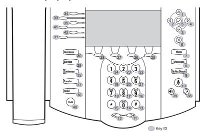
Note The SoundPoint IP 550 has only the top four lines keys.
